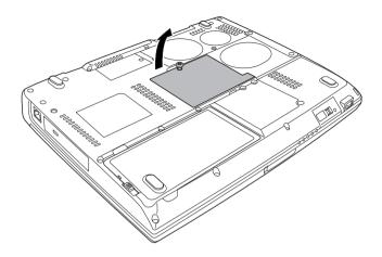
Figure 8-3 Removing the memory module cover
